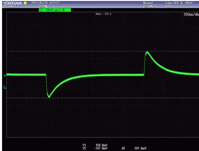
Measured Output Response to Step Load:
